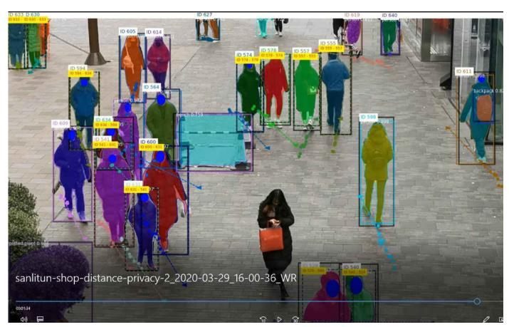
Privacy can also be active in tracking. Face and car plate extraction can also be provided as needed, and the results will be stored with the object ID for subsequent analysis.
